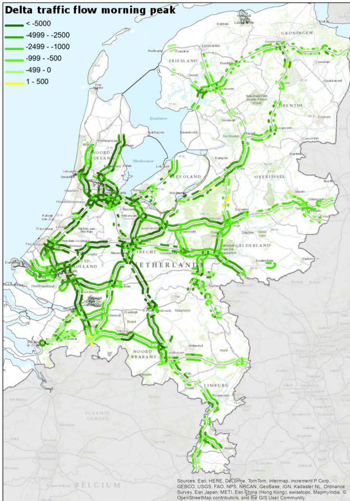
1 2 FIGURE 1 Change in traffic flows (vehicles per stretch per hour) on national roads in the 3 Netherlands by flexible working morning peak (6:00-10:00) in 2014, as compared to 2013.
