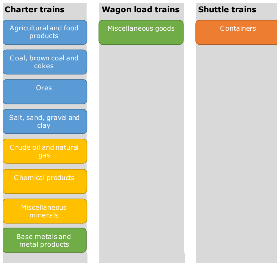
Figure 6.5 The three main functions of trains analysed for the railway transport mode and the commodity groups they transport. The colour scheme follows the same principle as in figure 2.1: blue signifies dry bulk, yellow signifies liquid bulk, green signifies break bulk and orange signifies containerized.
